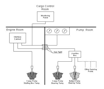
Figure 4-1 – Sample of temperature monitoring system
