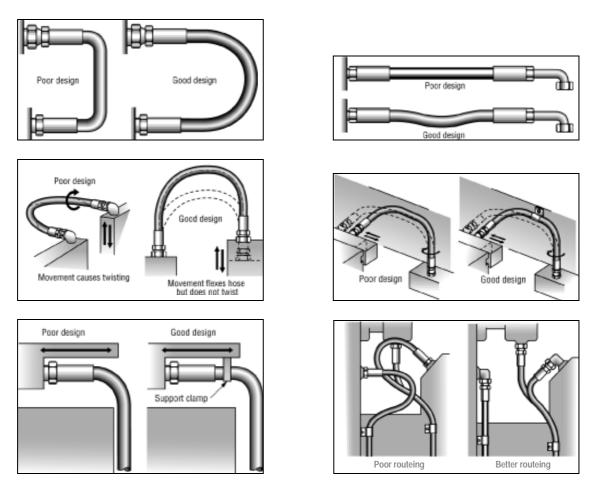
Figure 2-2 – Example of correct installation of flexible hoses
