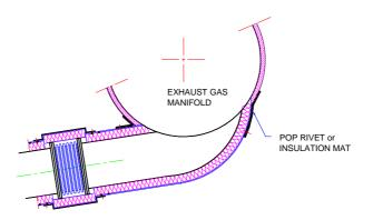
Figure 3-6 – Insulation practice of discontinuous part
