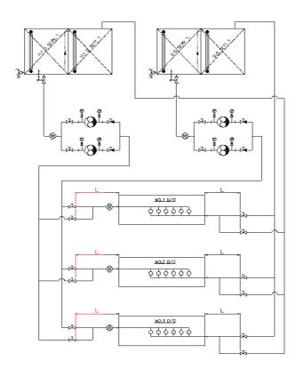
**Figure 3-10 – Acceptable arrangement of isolation valves**
