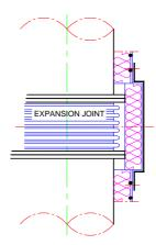
Figure 3-5 – Insulation method on compensator part
