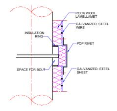
Figure 3-4 – Insulation method on flanged part
