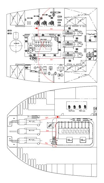
Figure 3-9 – Isolation valves arrangement for multi-engines
