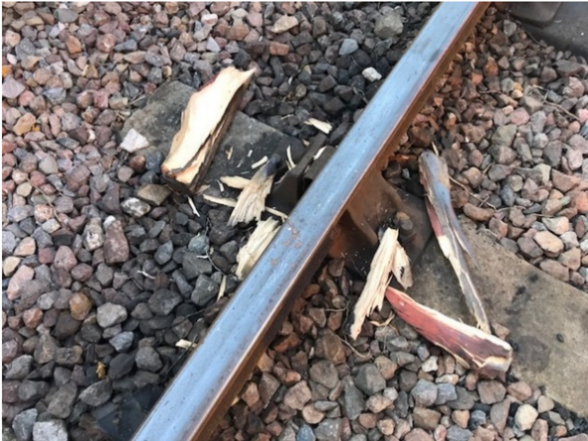
The remains of the destroyed chock (photograph courtesy of the Avon Valley Railway)
