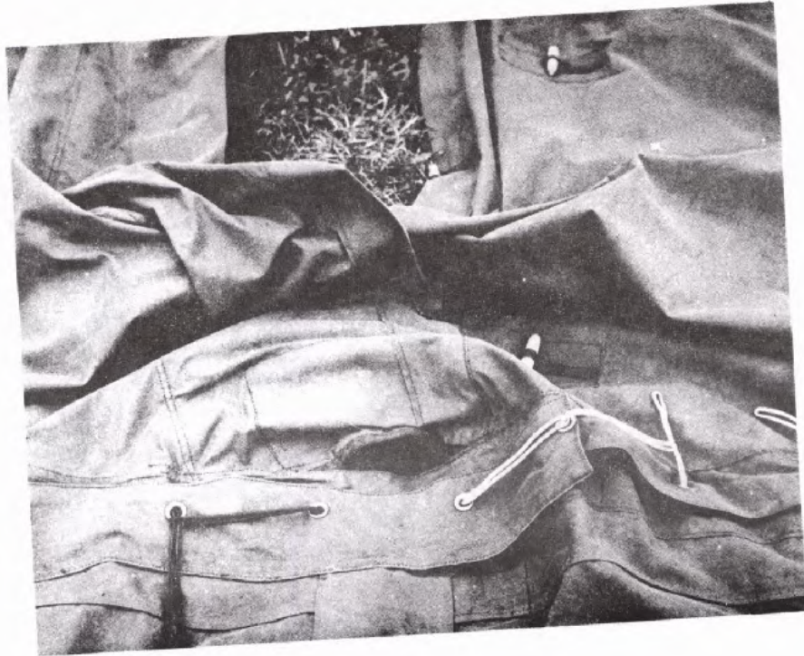
Fig 5 - Lay out covers, inside uppermost. Lace together, starting at the ridge.
