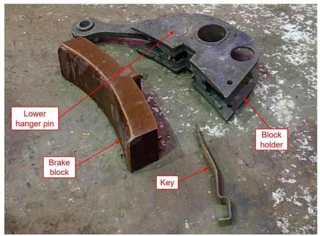
Figure 12: Block holder, key and brake block
