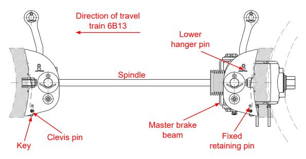
Figure 10: Side view of BFCB block holders (courtesy Wabtec Faiveley)
