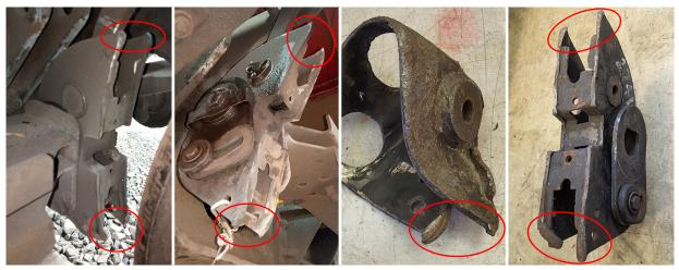
Figure D7: Brake block holders from wheel positions 8, 7 (both courtesy DB Cargo), 6 and 5 with worn corners indicated
