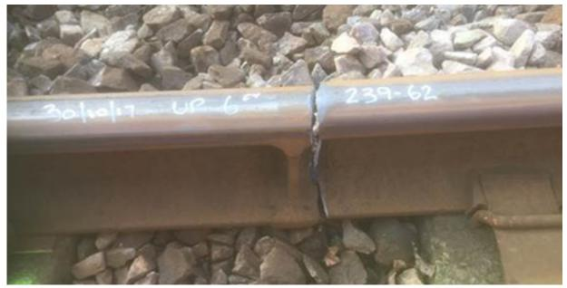
Figure 5: Broken weld 44.9 miles (72.2 km) from Robeston (courtesy Network Rail)
