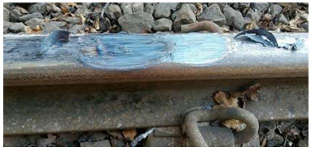
Figure 7: Damage to the rail head 67.2 miles (108.1 km) from Robeston (courtesy Network Rail)
