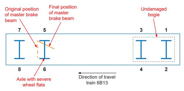
Figure D1: Schematic of wagon GERS89009 showing wheel numbering and the final position of the master brake beam
