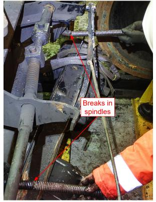
Figure D11: Reconstruction of bogie 2741; the visible part of the spindles would normally be hidden within the actuators mounted on the master brake beam (the detached brake beam is visible underneath)
