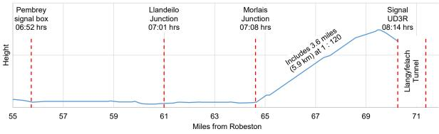
Figure 6: Gradient profile between Pembrey and Llangyfelach Tunnel
