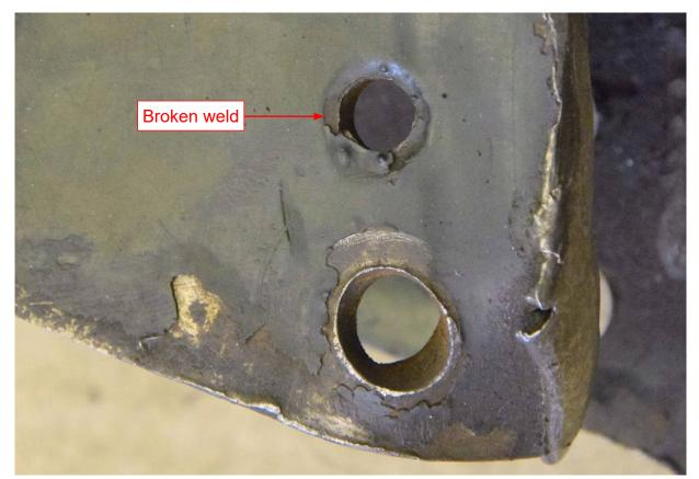
Figure 16: Inside corner of block holder from wheel position 5 (courtesy Serco Rail Technical Services)
