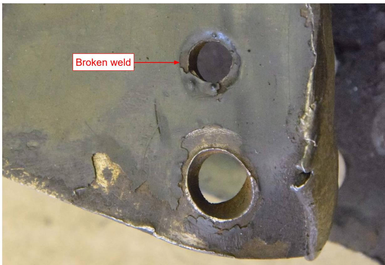
Figure 16: Inside corner of block holder from wheel position 5 (courtesy Serco Rail Technical Services)
