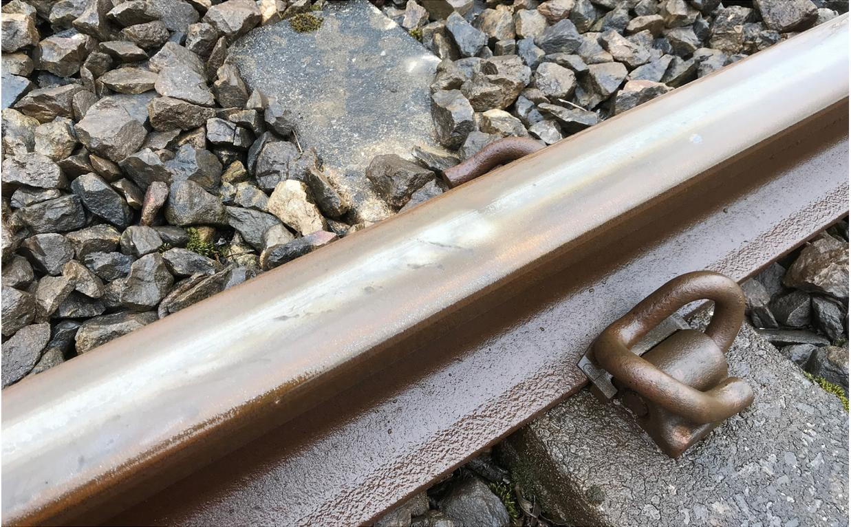
Figure 4: Rail head damage (six foot rail) 43.2 miles (69.5 km) from Robeston, still visible in April 2018
