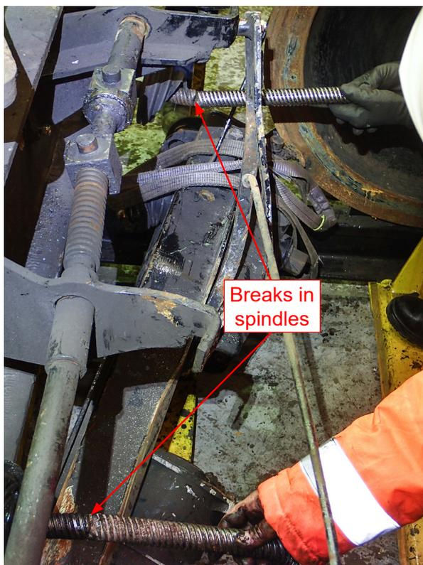
*Figure D11: Reconstruction of bogie 2741; the visible part of the spindles would normally be hidden within the actuators mounted on the master brake beam (the detached brake beam is visible underneath)*
