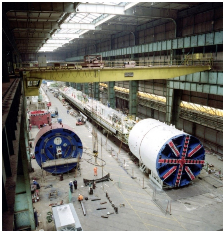
Figure 30: Photograph of a typical tunnel boring machine
