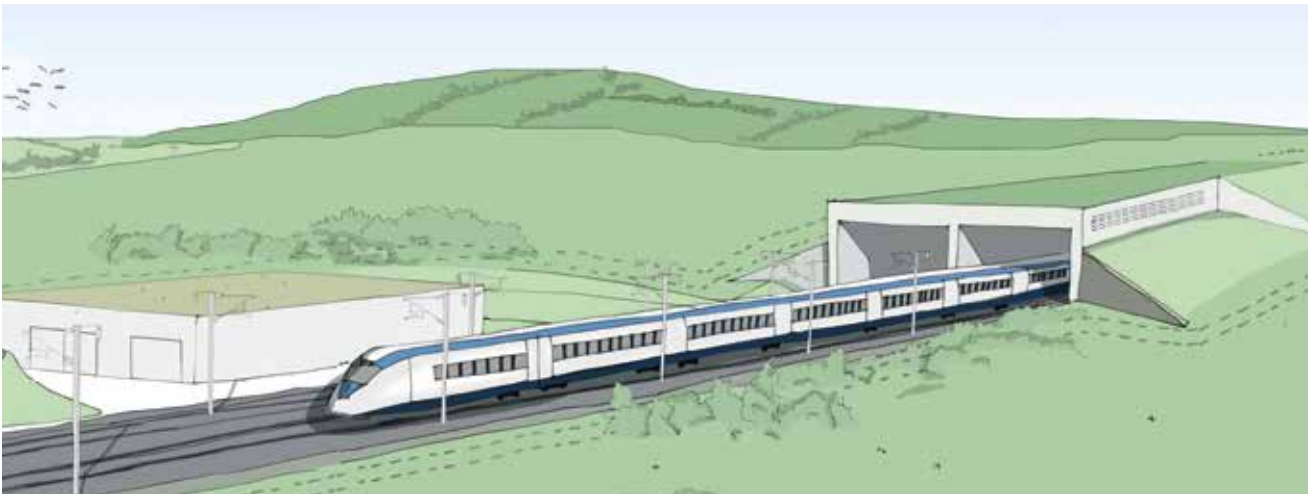
Figure 7: Illustration of cut-and-cover tunnel portal
