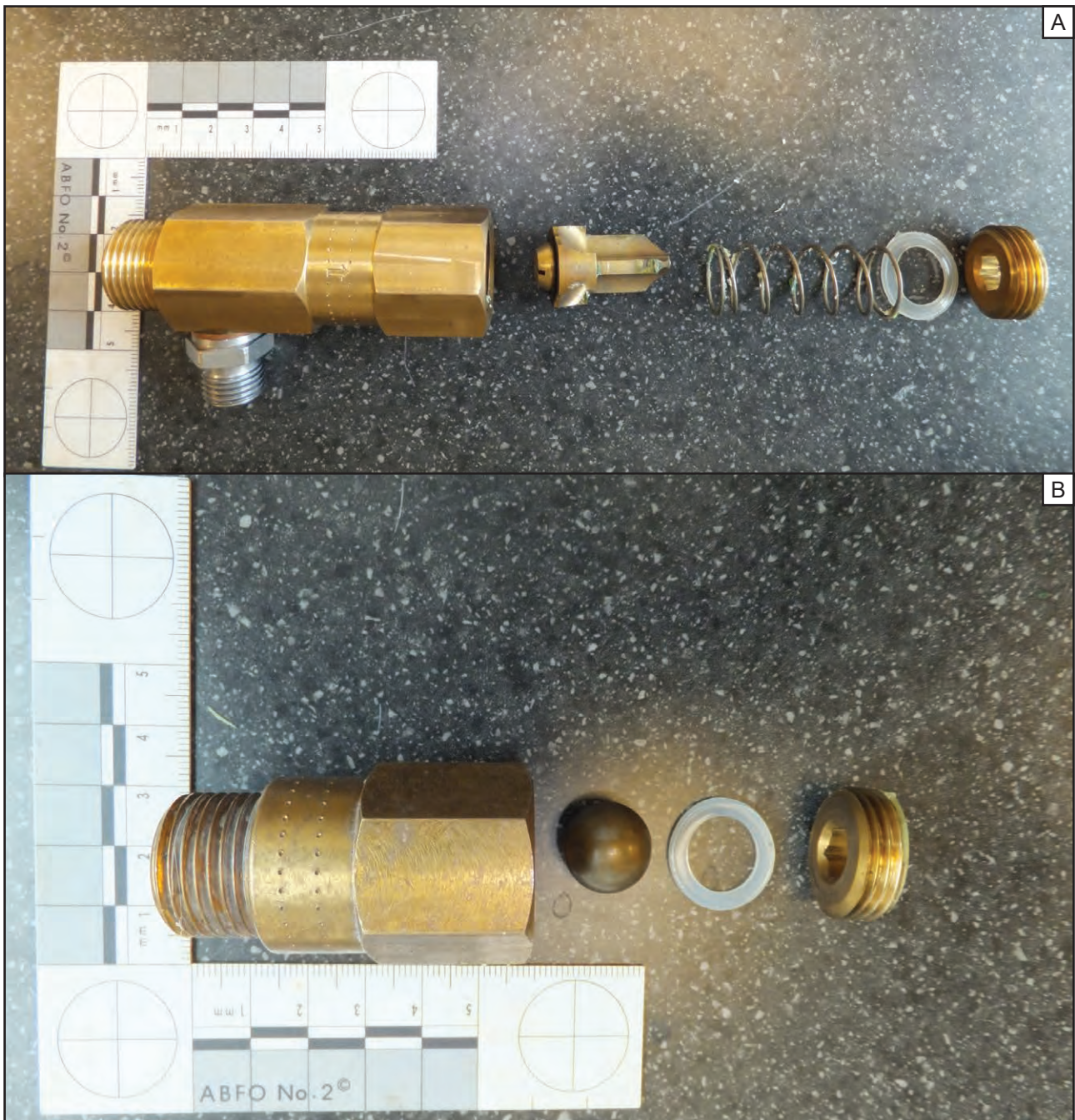
Figure 7: Non-return valve (A) and check valve (B)
