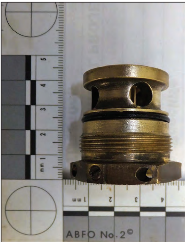
Figure 12c: Evidence of cleaning with wire wheel
