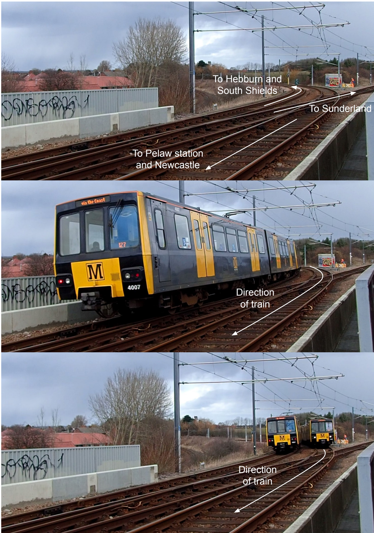
Figure 6: Images taken from the approximate location of the lookout at the time of the incident. It can be seen how an inbound train (second image) obscures the view of an oncoming outbound train (visible in third image).
