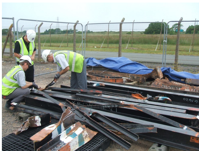
Figure 12: Metal waste being sampled before sentencing and disposal
