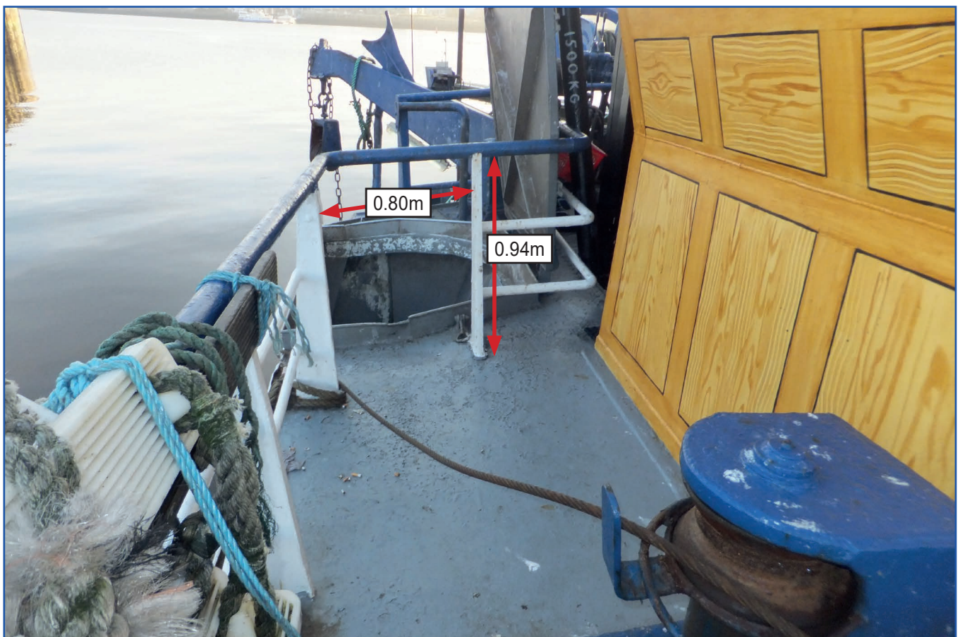
Figure 2: Illustris's guardrails and trawl wire gap dimensions
