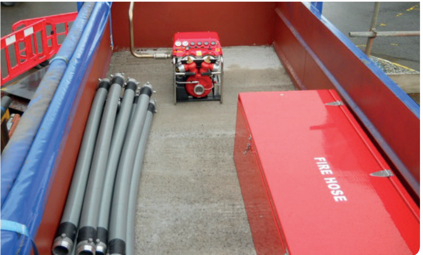
Figure 10: Diverse Flood Resilient Boiler Feed Pump at Oldbury
