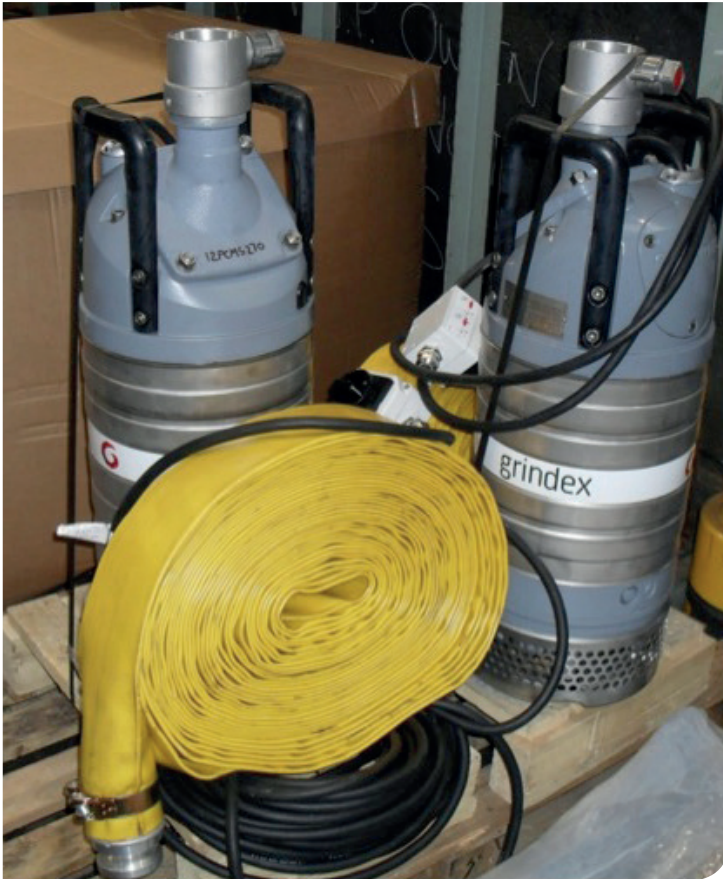
Figure 7: Submersible Pumps at Wylfa
