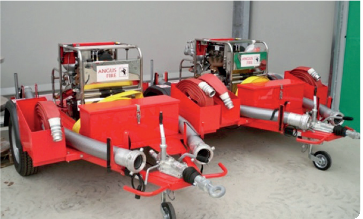
Figure 3: Diesel Driven Fire Pumps at Wylfa
