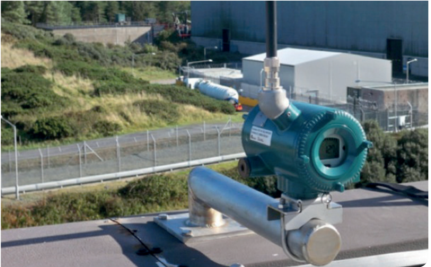
Figure 6: Alternative Emergency Reactor Monitoring System at Wylfa
