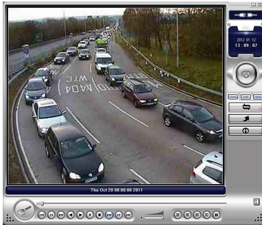
Figure 4.13 – Underutilisation of lane 3 on A404 Northbound approach to roundabout
