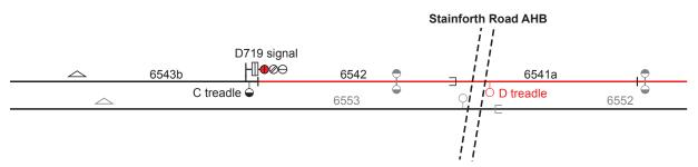
Figure 12: A train on the Down Skellow line operates Treadle D as it exits the crossing
