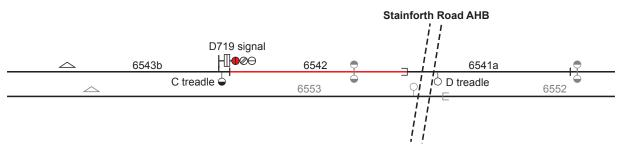
Figure 10: A train approaching on the Down Skellow line clears track circuit 6543b and occupies track circuit 6542
