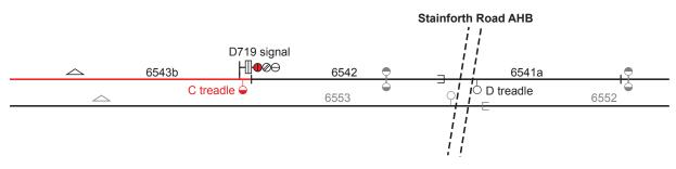
Figure 9: A train approaching on the Down Skellow line operates Treadle C
