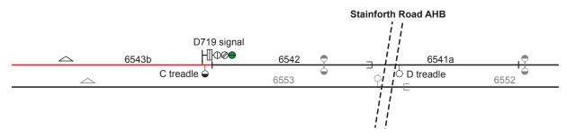
Figure 8: A train approaching on the Down Skellow line occupies track circuit 6543b
