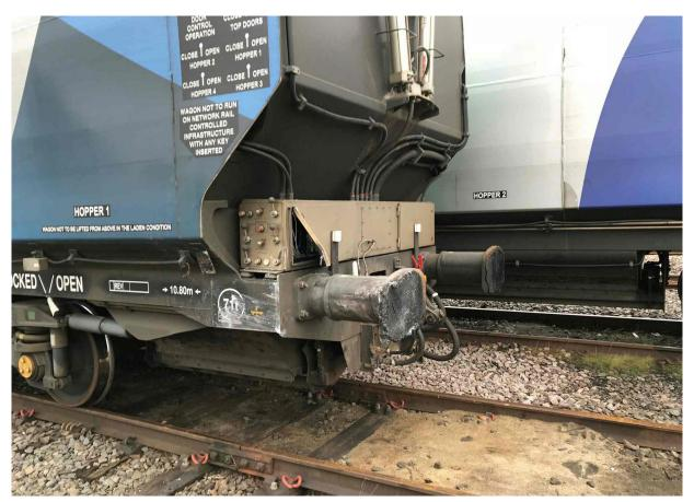
Figure 7: The damage sustained by the rearmost wagon as a result of the accident (image courtesy of Network Rail)
