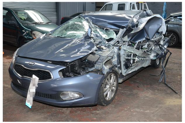
*Figure 6: The damage sustained by the car as a result of the accident (image courtesy of the British Transport Police)*
