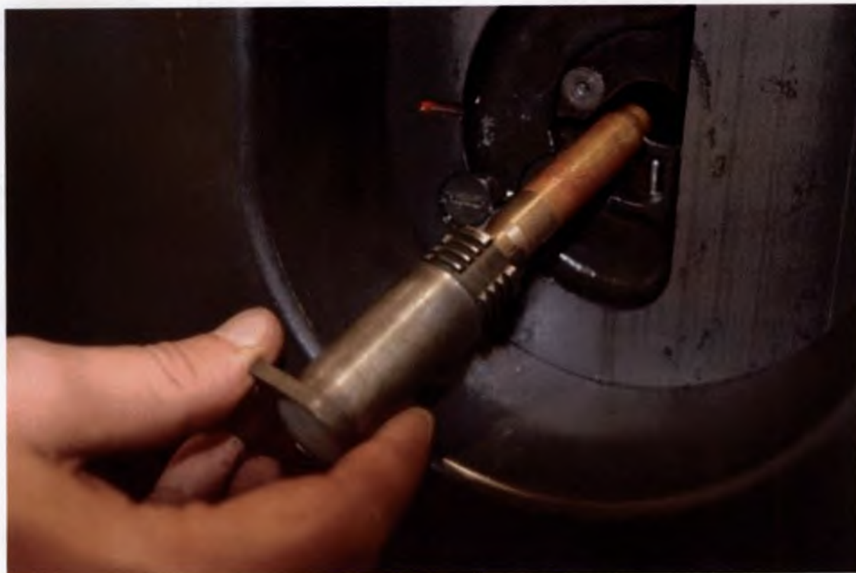
Figure 1.4.35: Hand Loading a Firing Needle Assembly with a Tube Vent Electric Fitted
