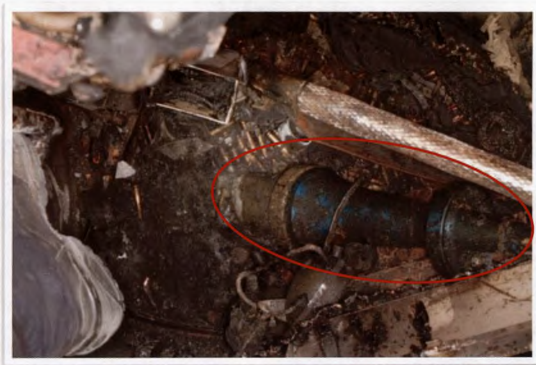
Figure 1.4.25: Discarding Sabot – Training Round on Tank Floor (circled in red) the ECBA has been removed
