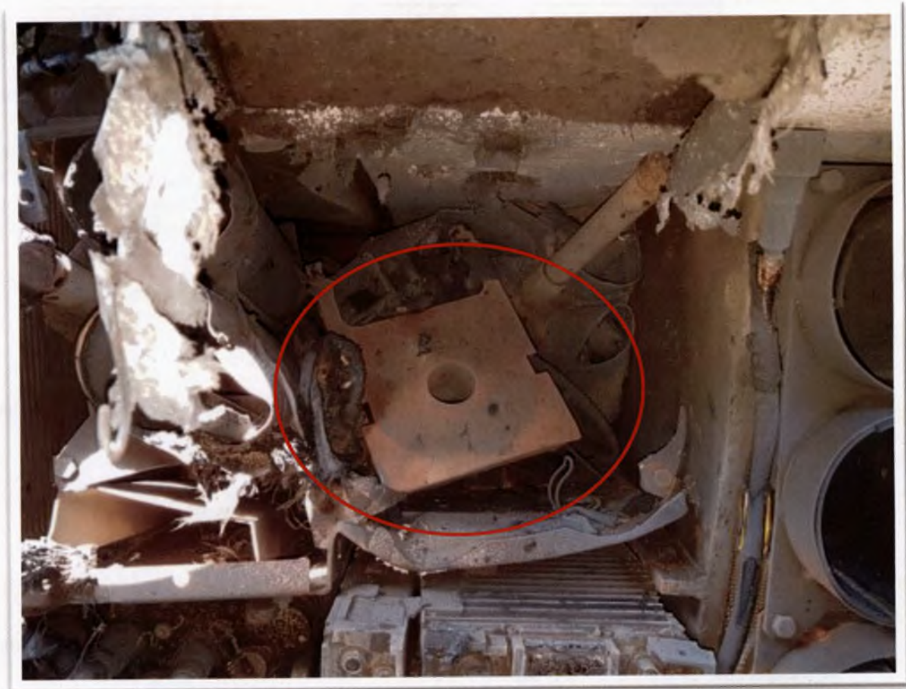
Figure 1.4.28: Upper Breech Block (circled in red) in the Projectile Racking
