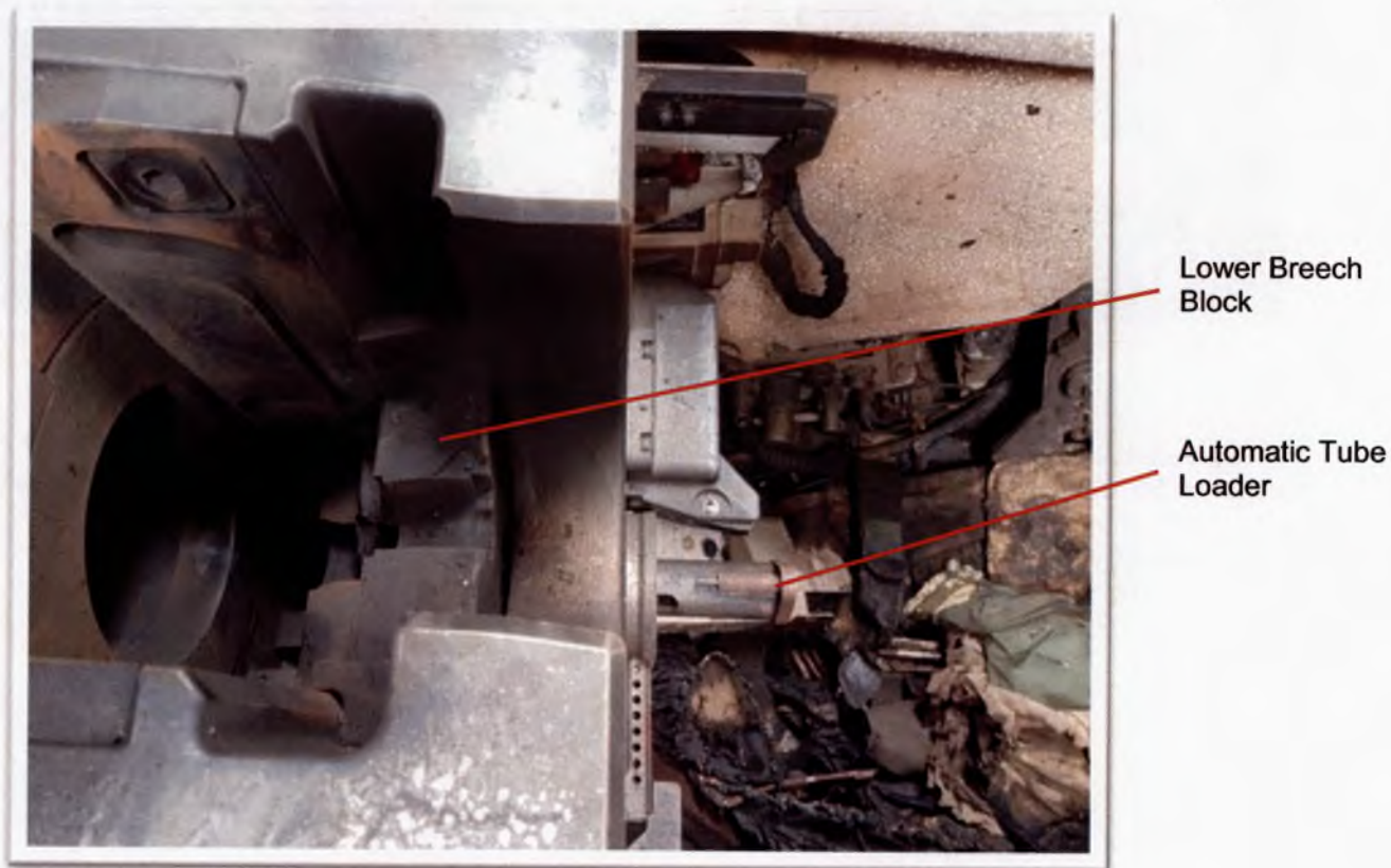
Figure 1.4.27: Damaged Breech Ring with Upper Breech Block Missing
