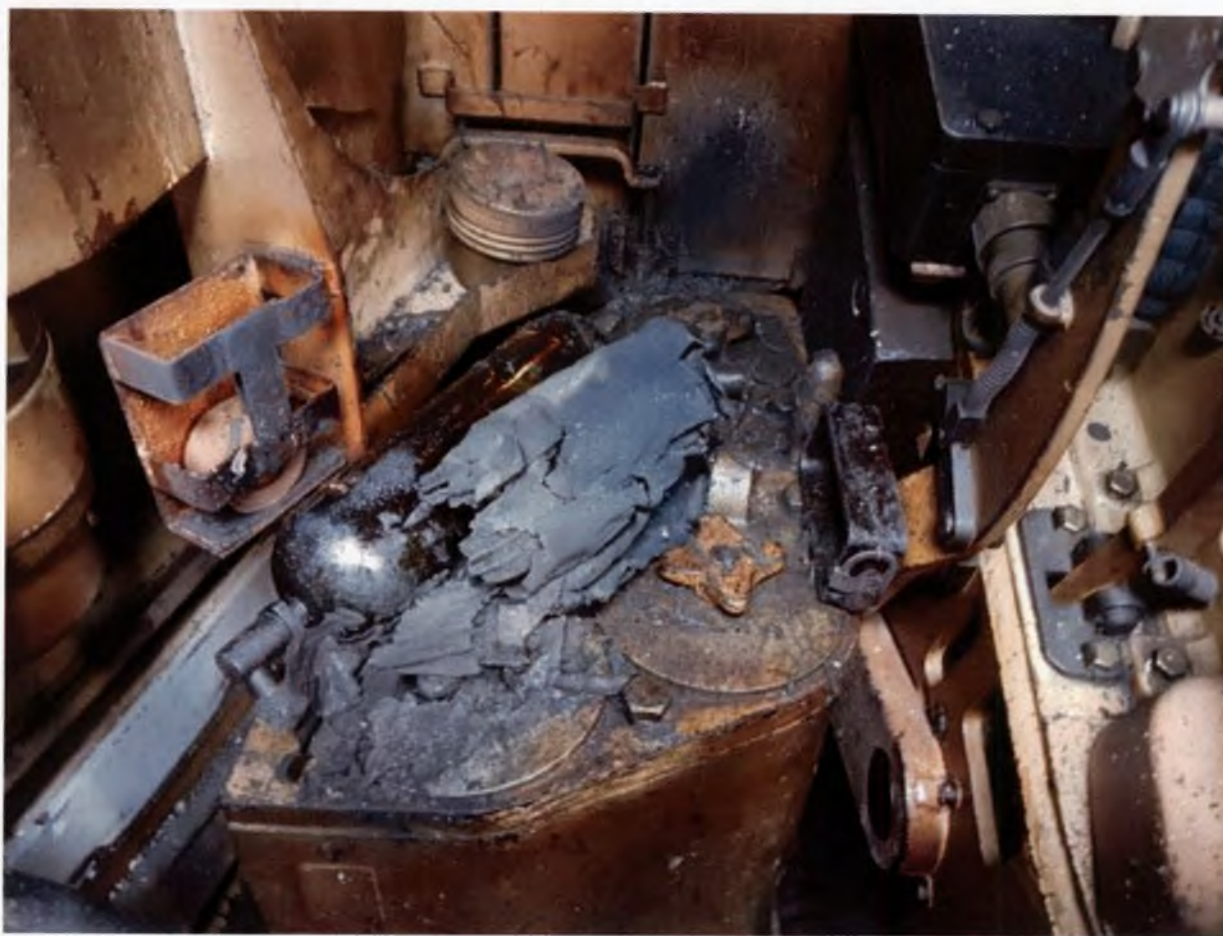
Figure 1.4.45: Post-Accident View of the Ready Charge Bin
