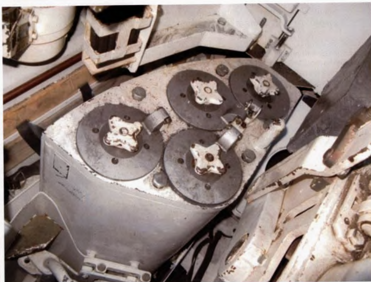
Figure 1.4.44: The Ready Charge Bin in a Reference Tank Each of the 4 stowages can hold one CP DS-T or 2 CP SH
