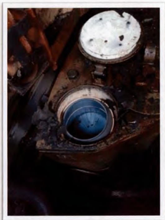
Figure 1.4.26: Remaining Charge Propelling Discarding Sabot – Training Left Photo: in the Charge Bin. Right Photo: as Recovered from the Tank
