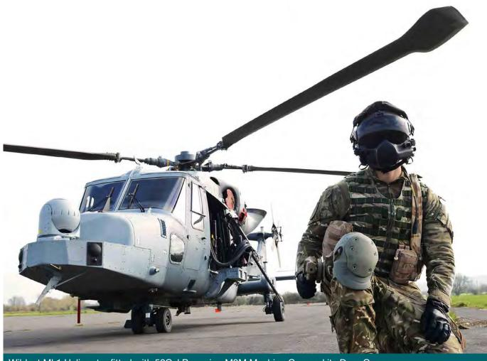
Wildcat Mk1 Helicopter fitted with 50Cal Browning M3M Machine Gun and its Door Gunner
