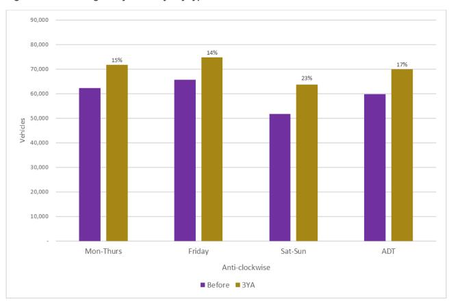
The overall AADT over the 12 months of Before and Yr3 After traffic data has increased by between 13% (J24-2J25 clockwise) and 18% (J26-J27 clockwise), with all the other sections/directions experiencing an increase in traffic flow of between 15% and 17%.
