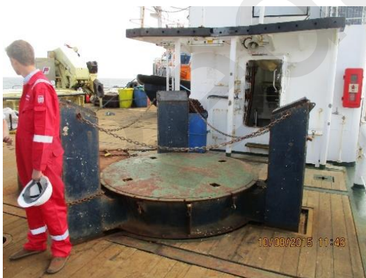
Figure 5: Buoy pod with 3 supporting pedestals - onboard Galatea
