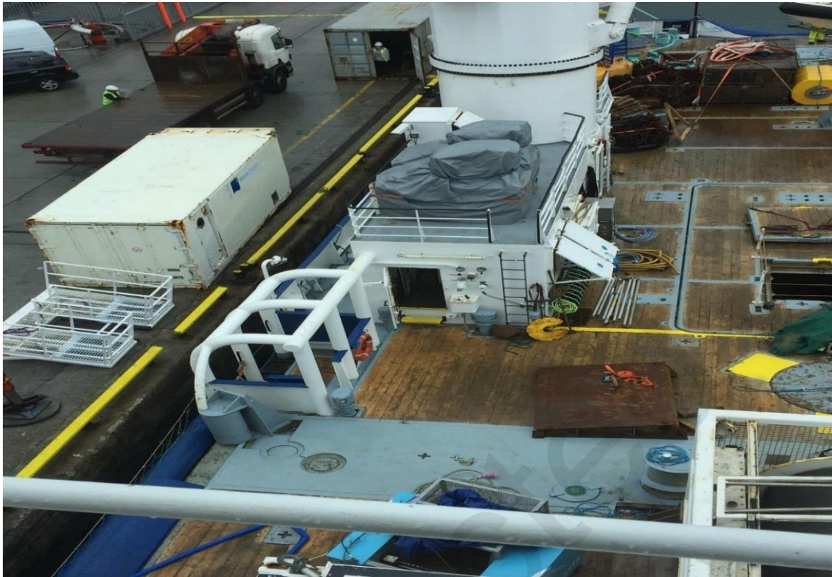
Photo 26 Note the fixed safety cage which the crew use during buoy recovery and laying operations.
