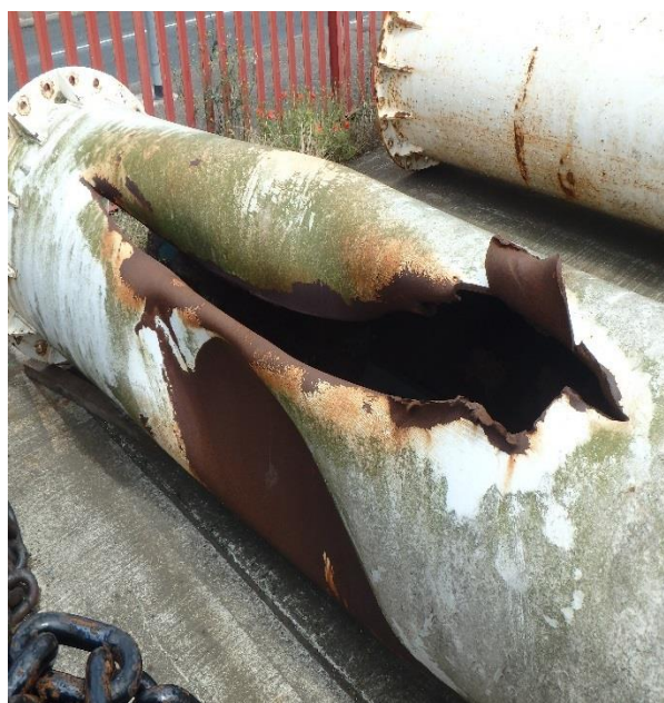
Photo 37 Buoy tail tube damaged by propeller.
