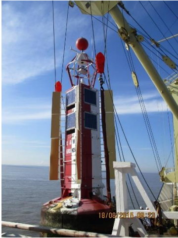
The Buoy located in a cradle on deck and ready to have the electrical system checked by a member of ship's staff
