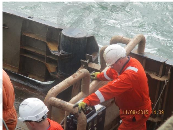
Operation of the chain holding equipment – a guillotine
