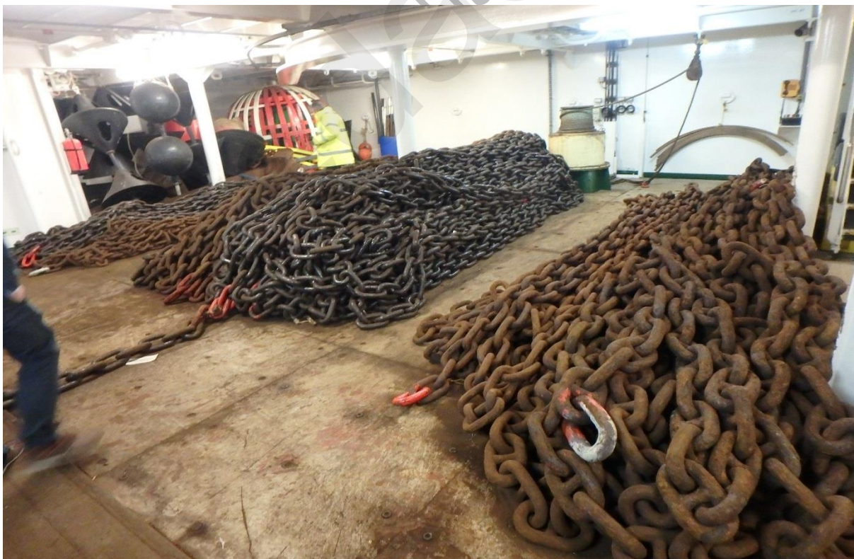
Photo 11 Substantial amount of neatly stowed chain in the storage hold. TPVs such as an AHTS are equipped with chain lockers for storage but the chain link size of 38 mm now uniformly used by the GLAs is not compatible with the much larger gypsies normally carried on board of these vessels. TPVs would also not carry spare amounts of this size of chain
