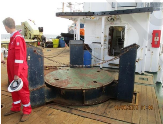
Area for storing Type 1 Buoy. Note the good condition of the working deck
