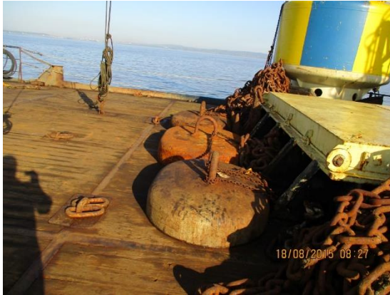
Two sinkers on the working deck ready for deployment when required
