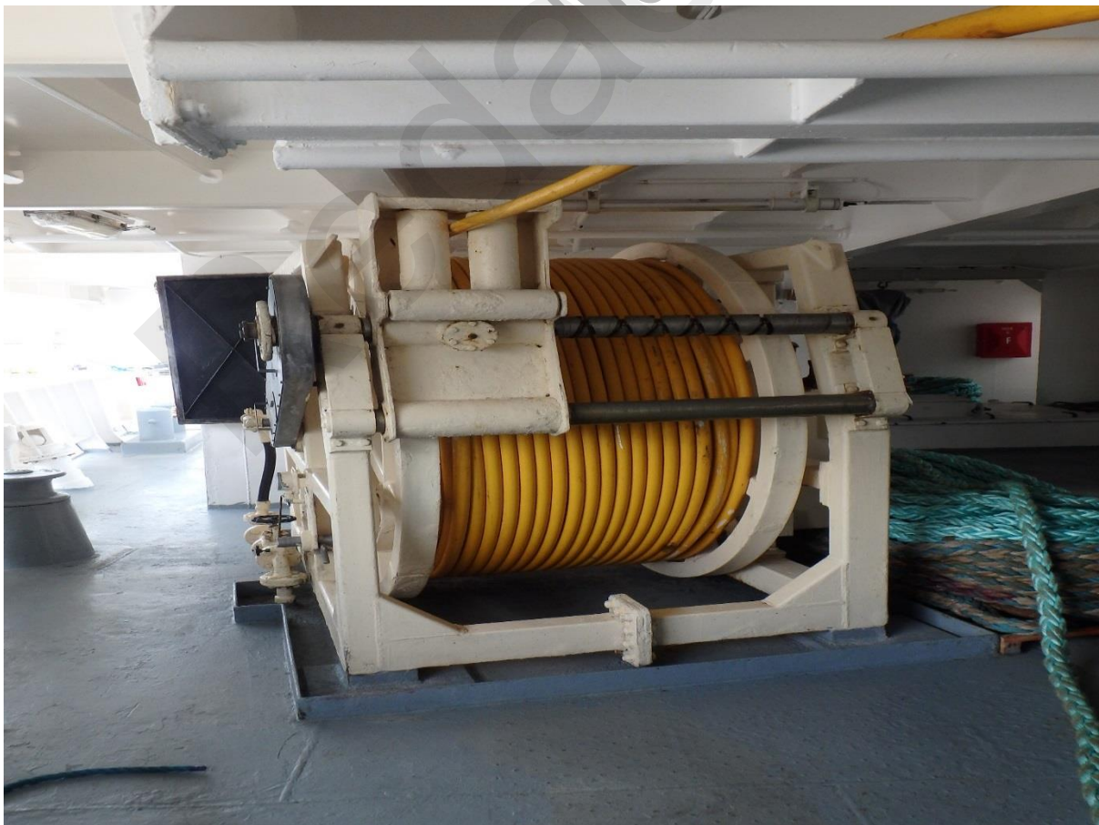
Photo 29 Water hose for supply to remote locations.
