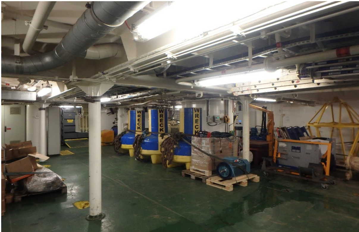
Photo 10 Large under deck storage hold with three Type 3 wreck marking buoys stored. Note that everything is neatly stowed and arranged. Most vessels such as AHTS on the GVCM would not have this large under deck storage area and would need spare buoys loaded on deck.
