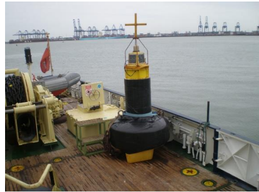
Type 3 Buoy on deck covered in black plastic to stop the UV
