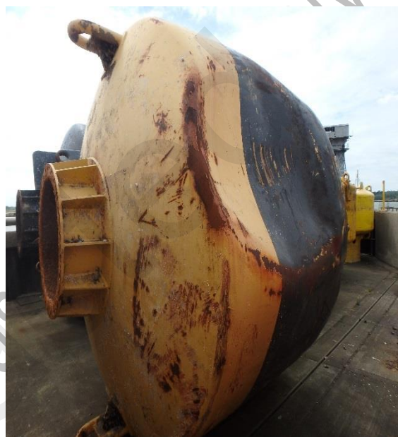
Photo 38 Buoy damaged in collision.
