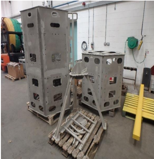
Photo 39 New Aluminium (LAS) top structures under construction.
