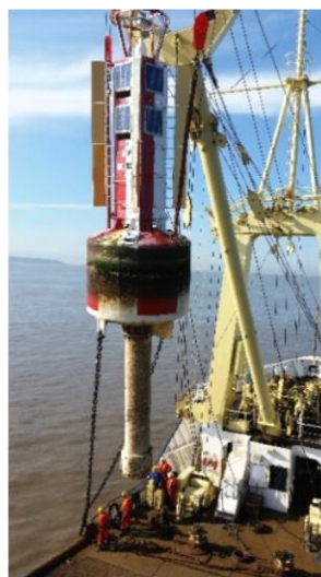
Figure 6: Type 1 Buoy being lifted onto Patricia's deck
