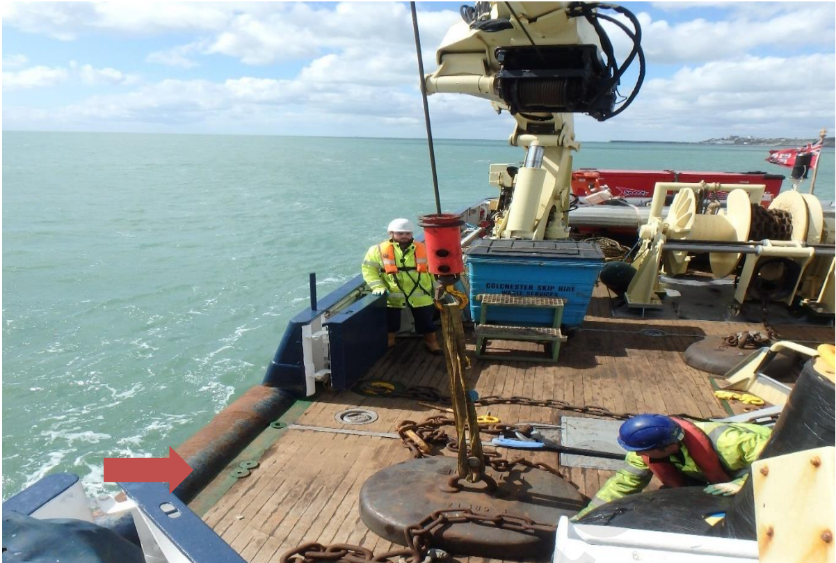
Photo 15 Sinker on deck about to be lifted over the bolster (arrowed).
