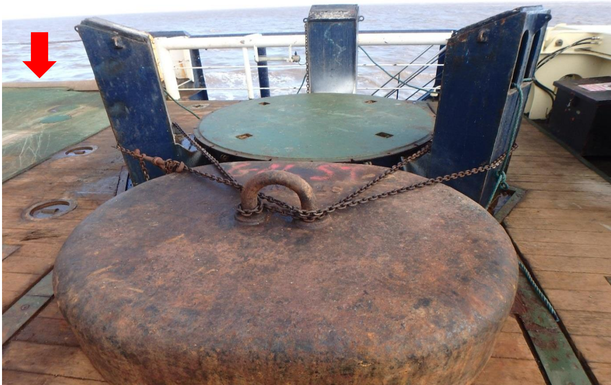
Photo 8 Closed pod with spare buoy sinker safely fastened down. The bolster (arrowed) can be seen in the top left.
