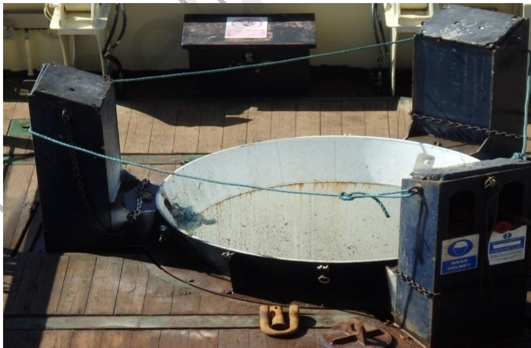
Photo 7 Close up view of the open pod showing the three buoy supports. Talking with some of the crew, they said that having four supports for the buoys as were on Patricia was better than having only three as on Galatea as it made for easier positioning of the buoys especially for a Type 2 buoy
