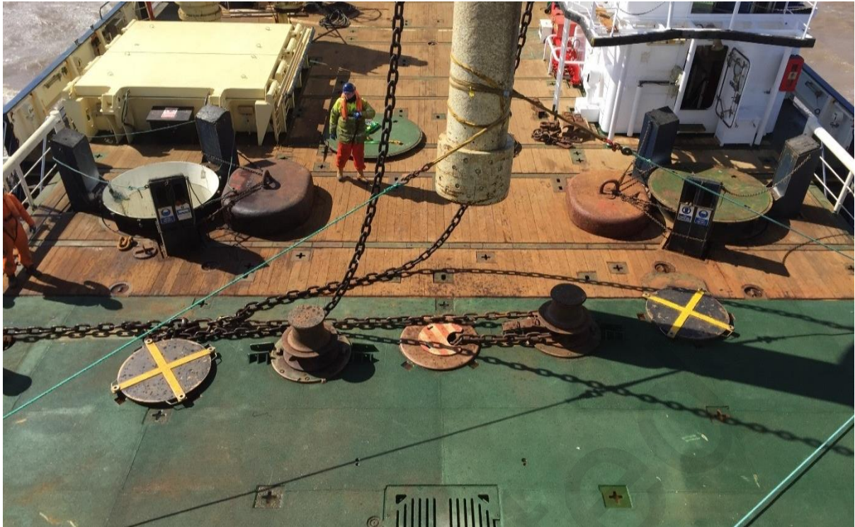
Photo 4 Buoy chain being retrieved with chain going around the gypsy and into the chain locker in the centre.
