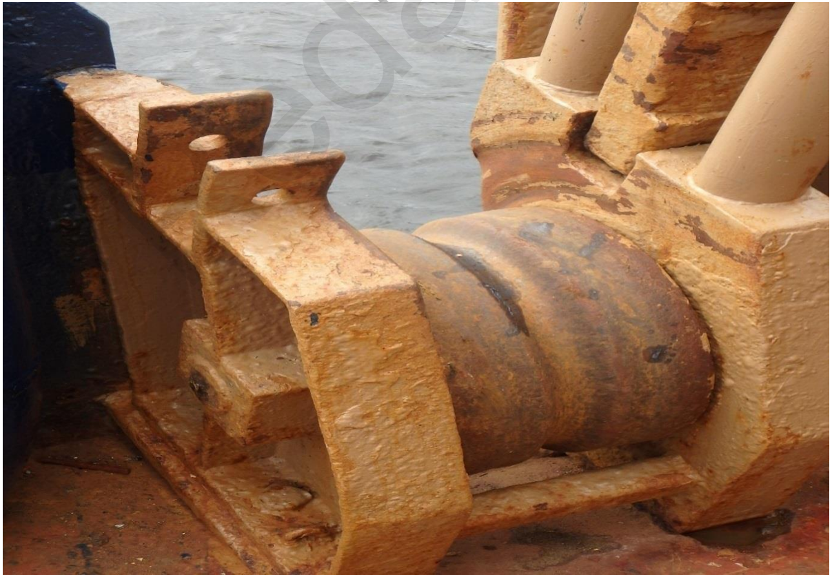
Photo 21 Roller for bringing the buoy chain on board.
