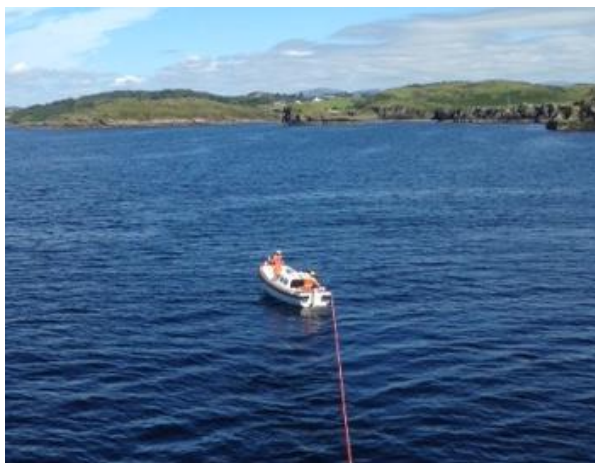
Figure 12: Fuel and water hoses being towed ashore for lighthouse replenishment from Granuaile
