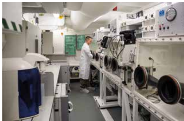
© Thales UK. Inside the laboratory of the new Thales Biological Surveillance and Collector System, designed to protect UK's deployed forces from biological attack by detecting incoming attacking particles in the air through specialised sensors and evaluating equipment. The system was designed by Thales, in partnership with Dstl, DE&S and 26 UK-based suppliers including 17 SMEs.
