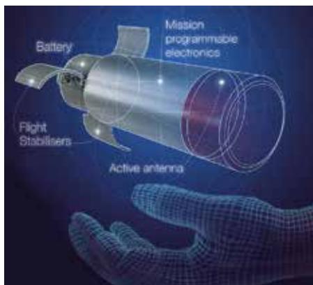
BriteCloud Miniature Missile Decoy Packed with missile-confusing advanced electronics.
