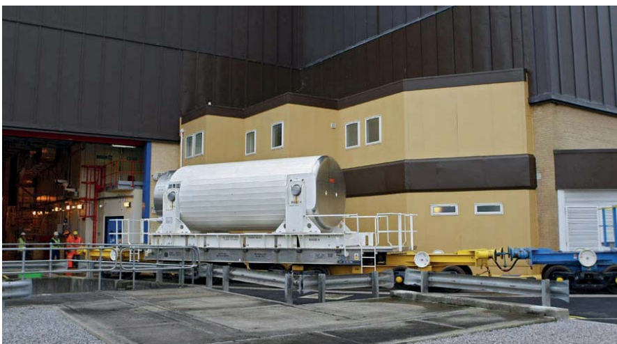
Top Left: Vitrified containers stored in our 8,000 capacity store. Top Right: The Waste Vitrification Plant started operating in 1990. Bottom Right: Clean waste containers ready for export to the store. Above: A transport flask containing vitrified waste outside the Residue Export Facility, awaiting transportation to its country of origin.
