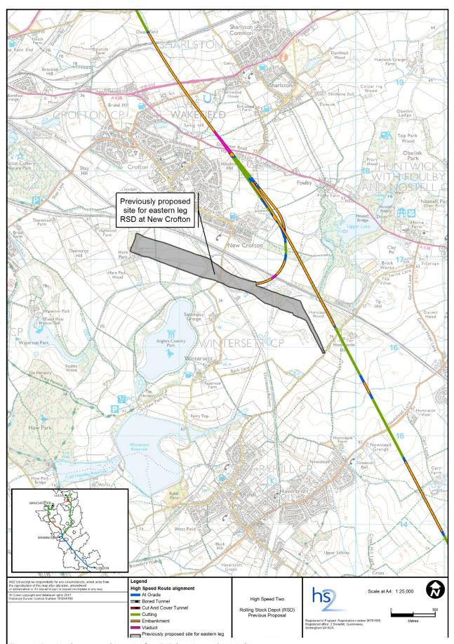
Figure 2: Previously proposed New Crofton RSD location and 2016 alignment
