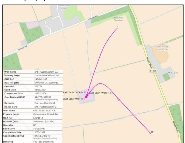
Site Plan 3: Trajectory of production wells at East Glentworth wellsite
