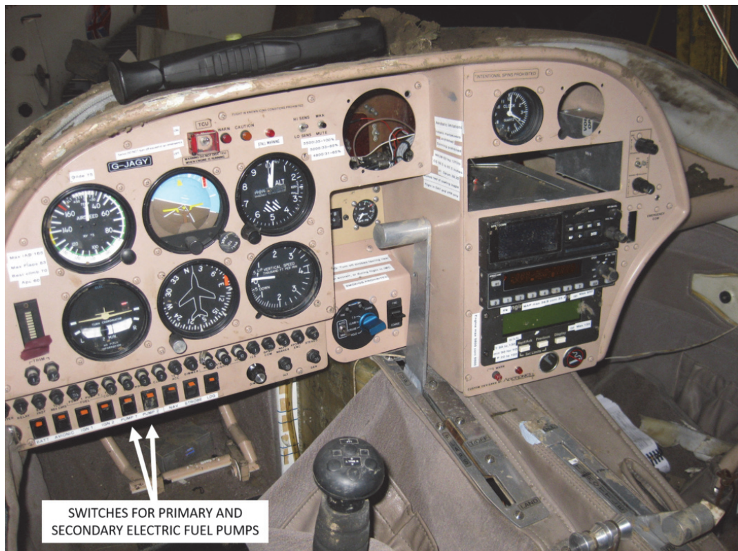
Figure 2 Fuel pump switches
