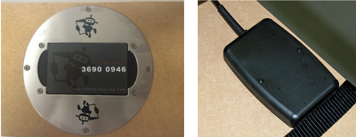
Figure 6 - Customer RFID card reader with RFID card and Controller iPad card reader
