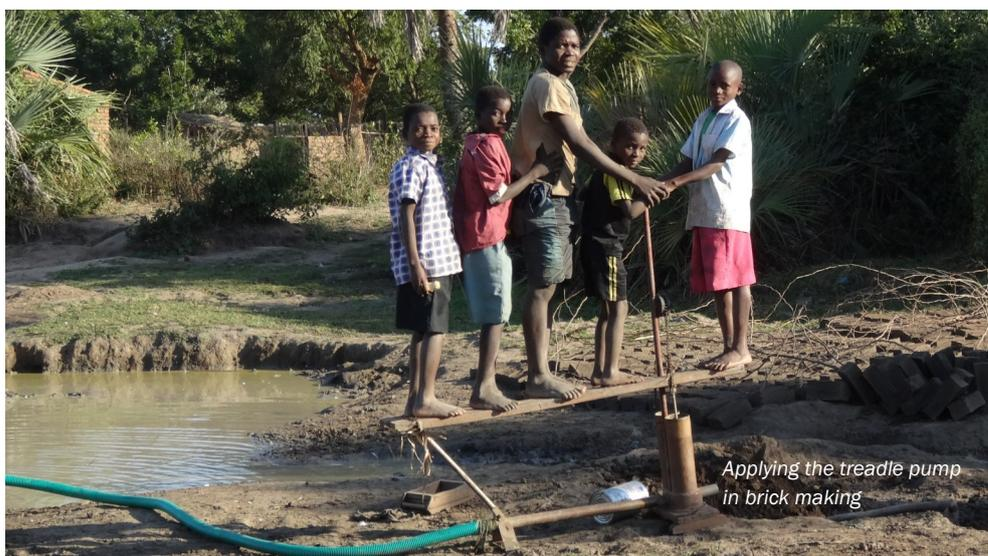
Applying the treadle pump in brick making
