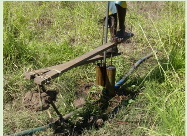
Farmers' innovation with the treadle pump has centred on making the treadle pump lighter to use and replacing spares by locally and cheaply available alternatives
