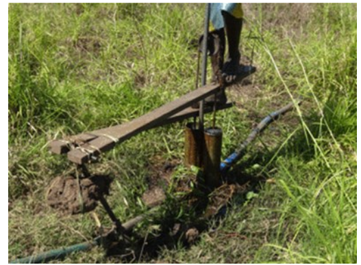
Farmers' innovation with the treadle pump has centred on making it lighter to use and replacing spares by locally and cheaply available alternatives.
