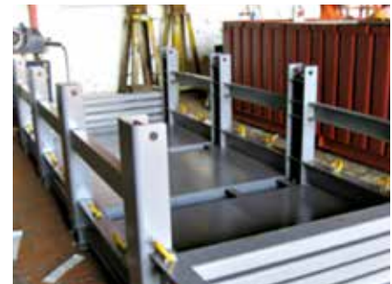
S2 full size stillage showing adjustable end bars
