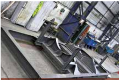
Specialised restraint system design, manufactured to restrain multi element bottles into TC01 package designs
