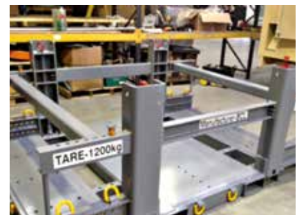
S3 half size stillage fitted with restraint bars for transportation of drums
