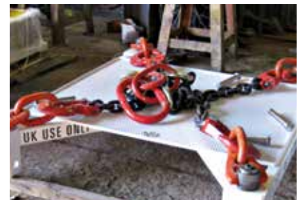
Stillage Lifting Frame (L2) which is compatible with both S2 and S3 stillages, and capable of a 27.5te lift
