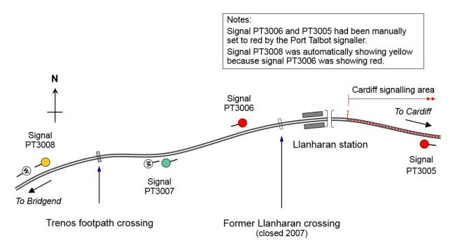
Figure 10: diagram at about 15:38 hrs
