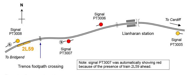
Figure 15: diagram at 15:51 hrs
