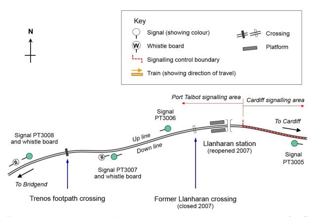
Figure 7: track and signalling layout diagram (not to scale). Note that the boundary between the Cardiff and Port Talbot signalling areas is staggered and signal PT3005 is within the Port Talbot signalling area.
