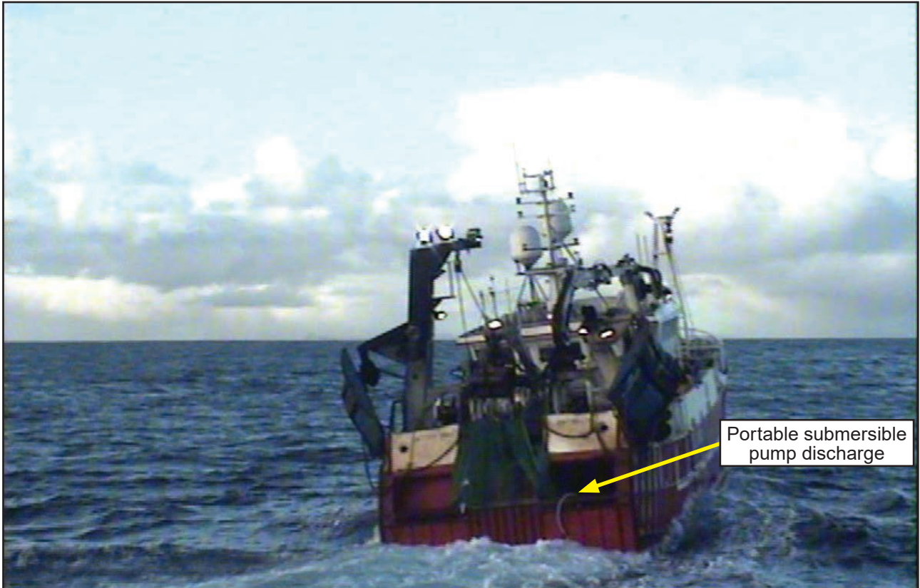
Figure 6: Ocean Way during the flooding with the submersible portable pump discharge visible on the starboard side
