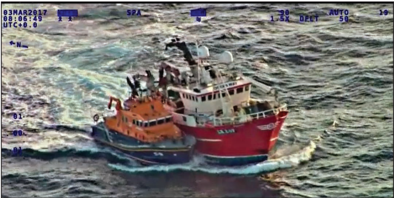
Figure 9: The Lerwick lifeboat alongside Ocean Way to transfer its salvage pump and two lifeboat men
