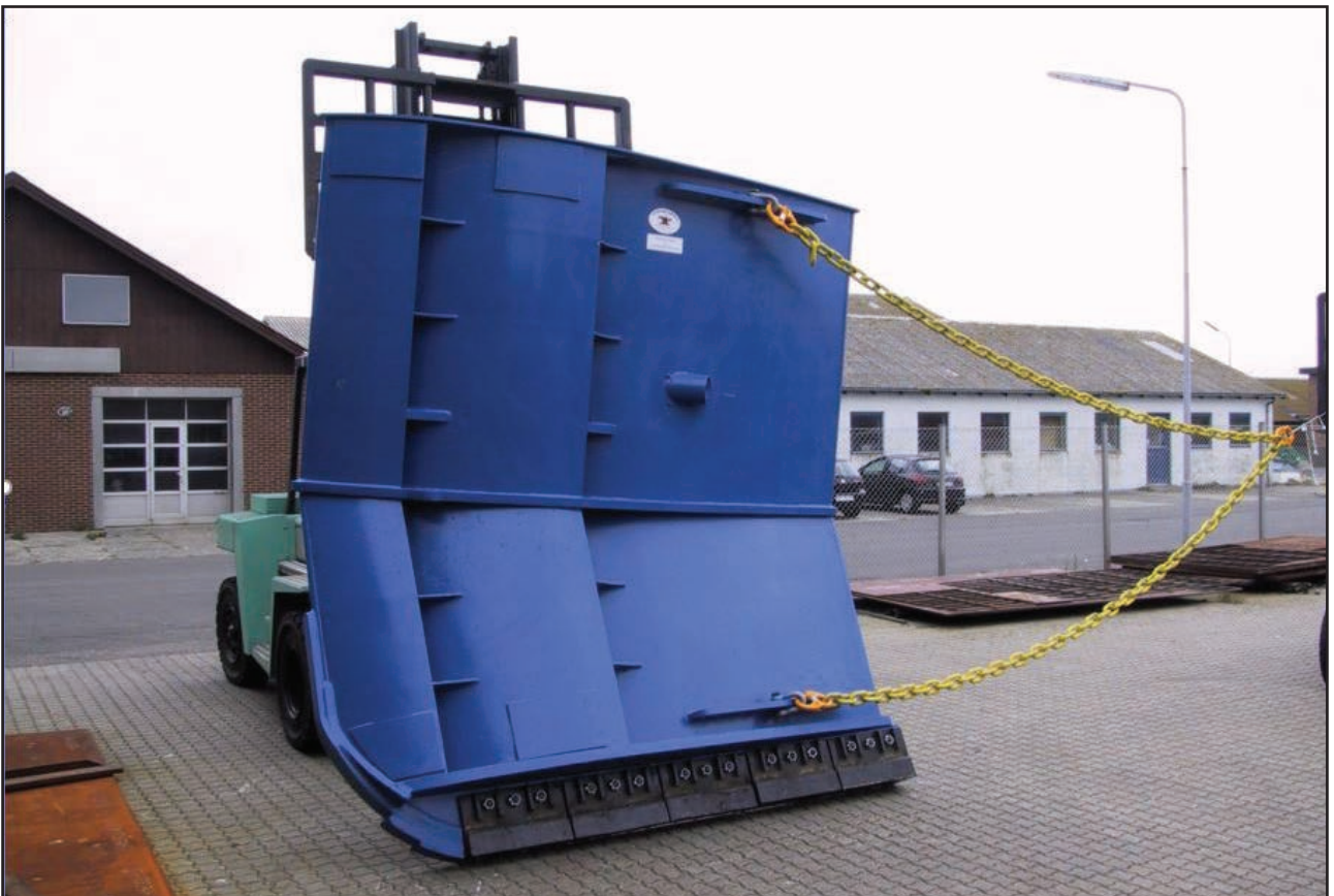
Figure 15: Thyborøn Type 12D trawl door
