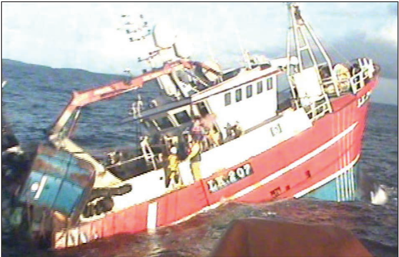
Figure 10: Ocean Way listing to port and trimmed by the stern just prior to foundering
