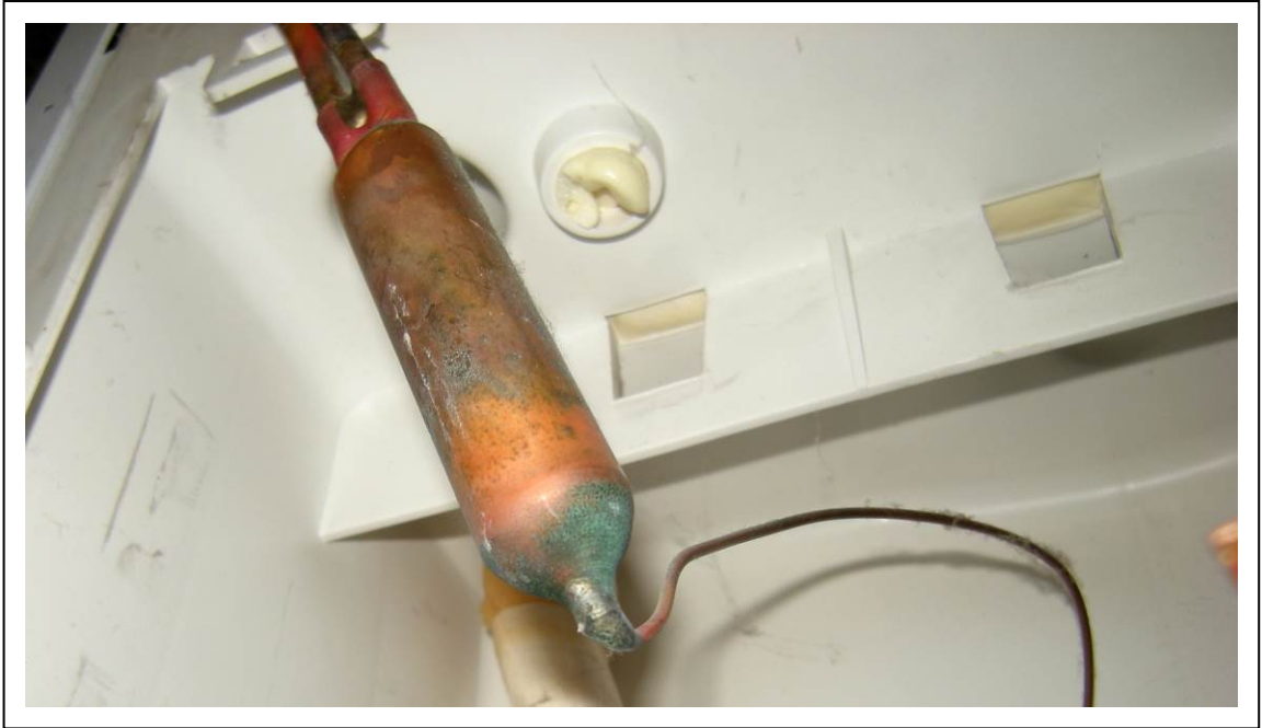
View of insulation foam visible at roof of compressor cavity
