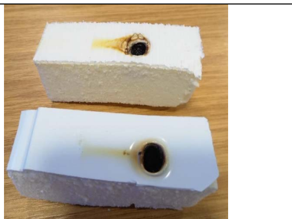
Photo 9 – Glow wire test on HB40 material and sandwich construction
