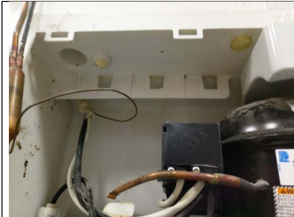
Photo 4 Compressor cavity, exposed foam at fill and vent point and behind cut-outs in web
