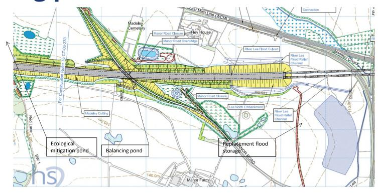
The image above shows how ecological mitigation ponds, balancing ponds and replacement flood storage areas are illustrated on the CT-06 maps.
