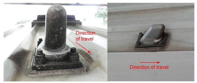
Figure 14: The radio antenna on the roof of the DVT (images courtesy of Arriva Trains Wales)
