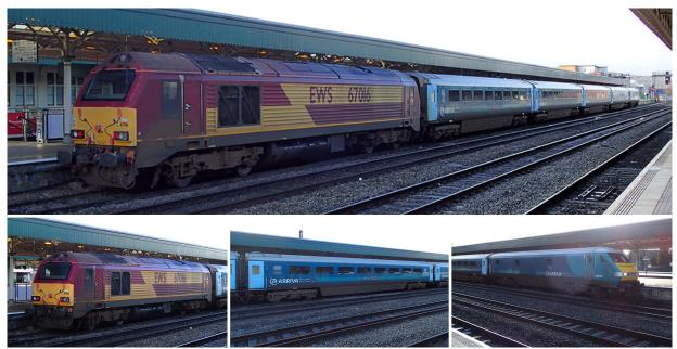
Figure 4: Class 67 locomotive, passenger coach and driving van trailer (DVT)
