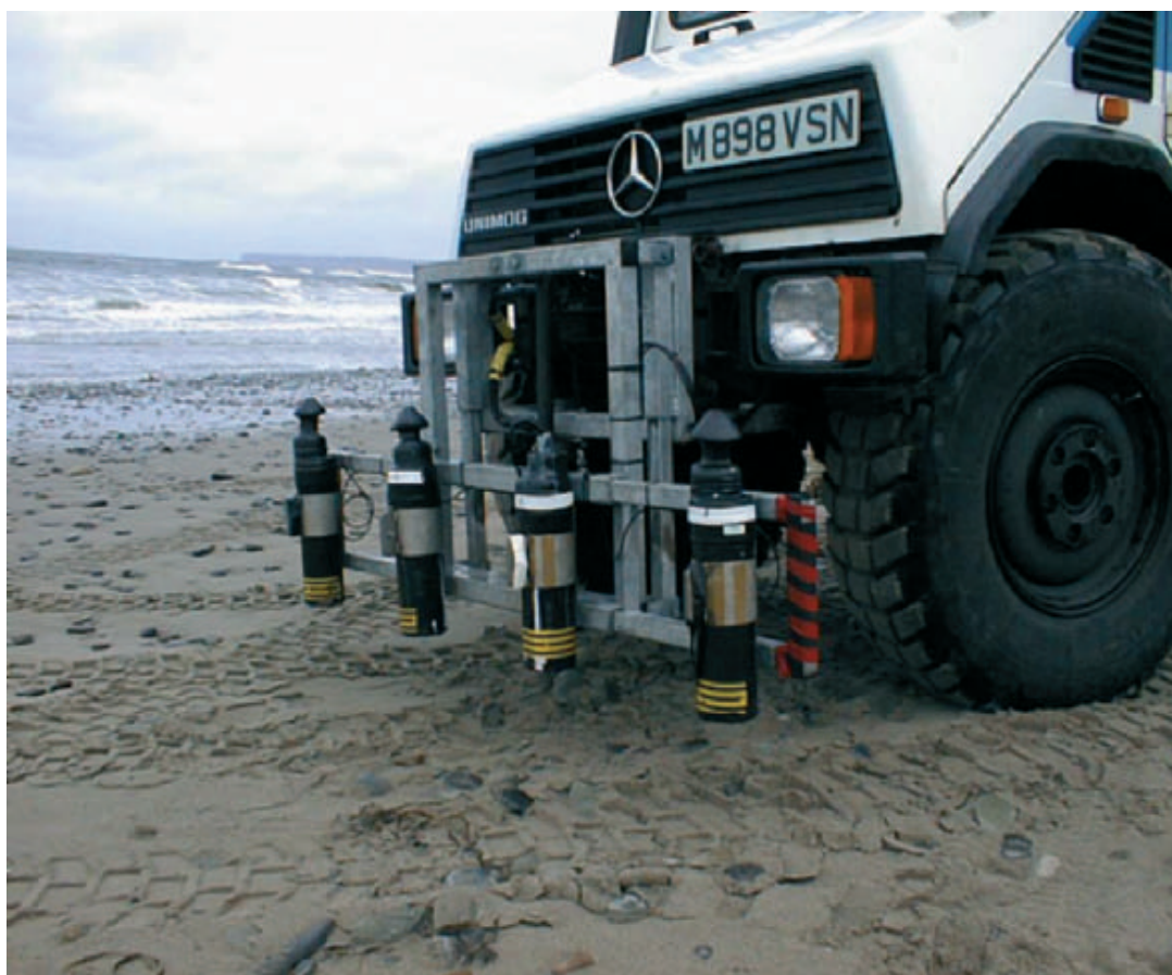
Figure 5.10 Groundhog Mk 1 system, with four 76 x 76 mm diameter NaI(Tl) Detectors
