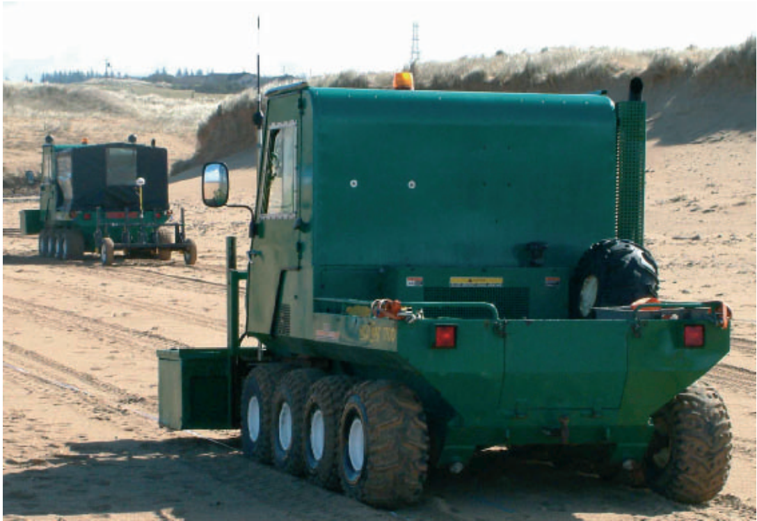
Figure 5.16 Example of Groundhog Evolution (pictured right) and the reconstructed Mk 1 system towed behind the first Hillcat (pictured left).
