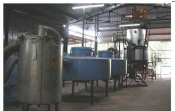
Decommissioned Ankur gasifier and filter line, Muzizi tea estate, James Finlay Uganda
