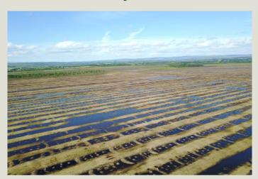
This aerial view of Bolton Fell Moss really shows the extent of the restoration work that has already taken place. The re-profiling works mean that the bog is now starting to hold water and vegetation is starting to grow back.
