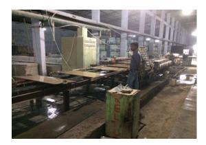
Normally, production continues 24 hours a day, 365 days per year. The owner forcibly stops production only for maintenance procedures – "the furnace has a temperature of 1,200 °C and requires three days to cool down and another three days to start up."
