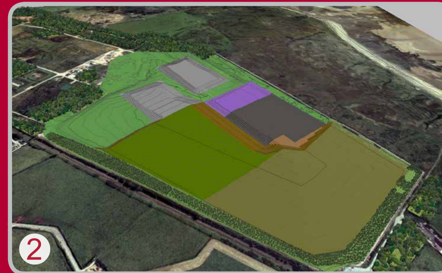
Phase 2 (2020 - 2022) – Capping of Vault 8 and adjacent Trenches, construct Vaults 9A and 10
