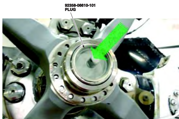
INSTALLATION OF PLUG FIGURE 11
