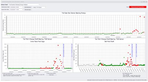
Figure 15 SGBA Tail Gearbox Bearing Energy Analysis Tool
