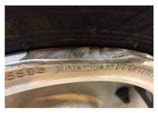
**Figure 17** Left outer wheel rim distortion (courtesy of CHC Scotia Ltd)
