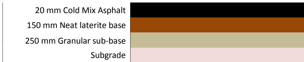
Figure 12-2: Designed pavement structure (E511)
