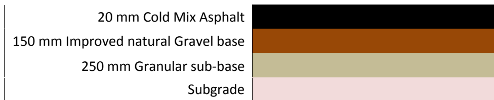
Figure 6-2: Designed pavement structure (D388)
