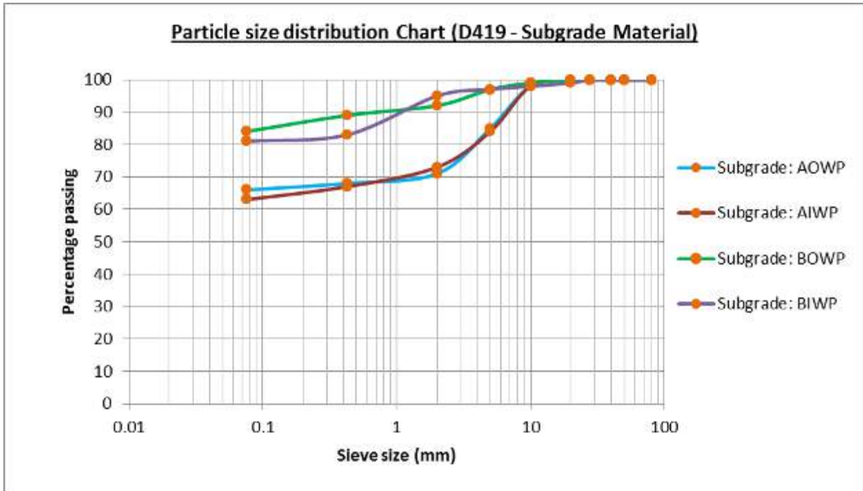
Figure 8-8: Particle size distribution chart for subgrade material (D419)
