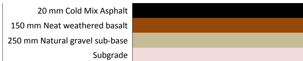
Figure 11-2: Designed pavement structure (D435)
