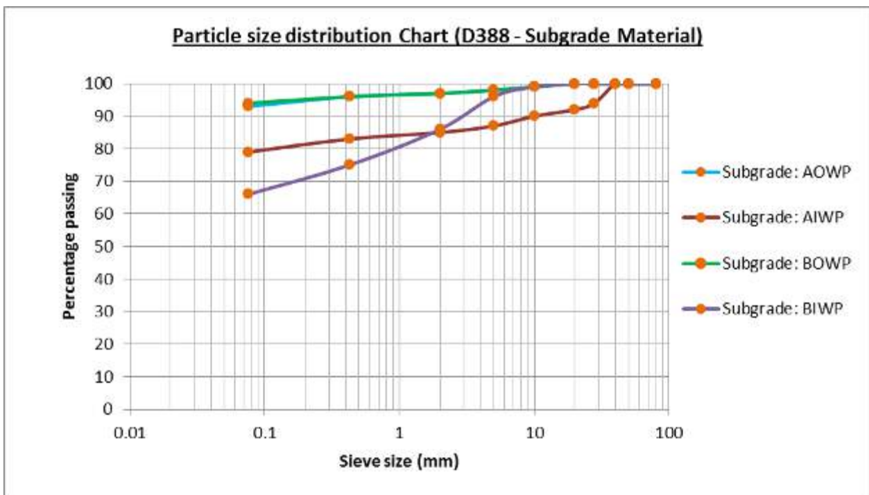
Figure 6-8: Particle size distribution chart for subgrade material (D388)
