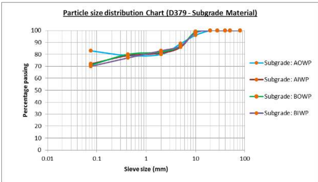
Figure 3-8: Particle size distribution of the subgrade material (D379)
