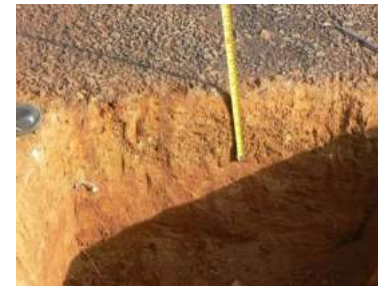
Typical 2-layer LVR pavement structure : Ntchisi (school) road
