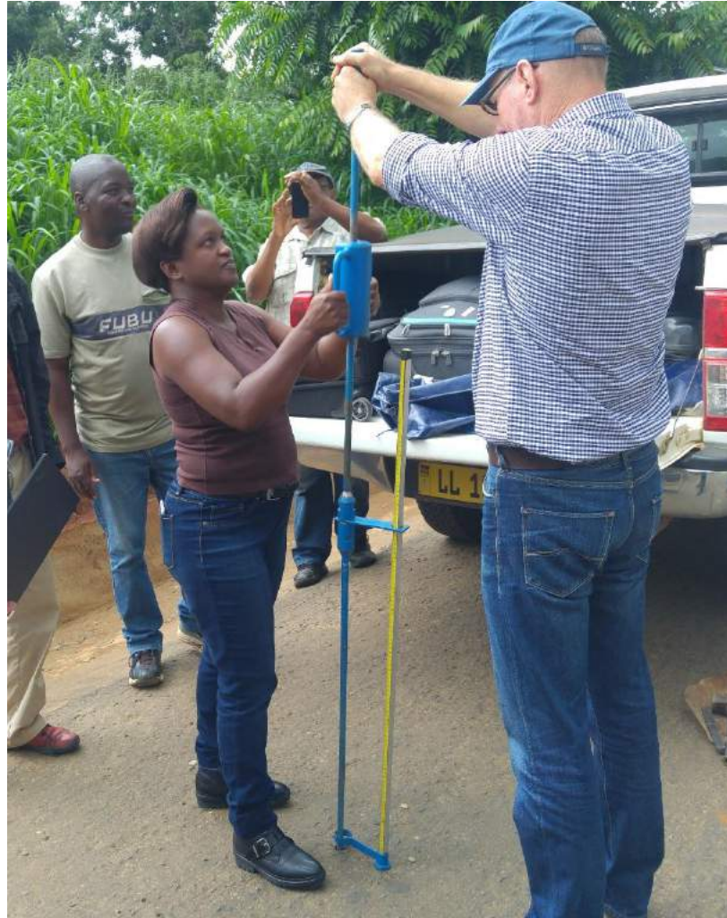
DCP test in process
