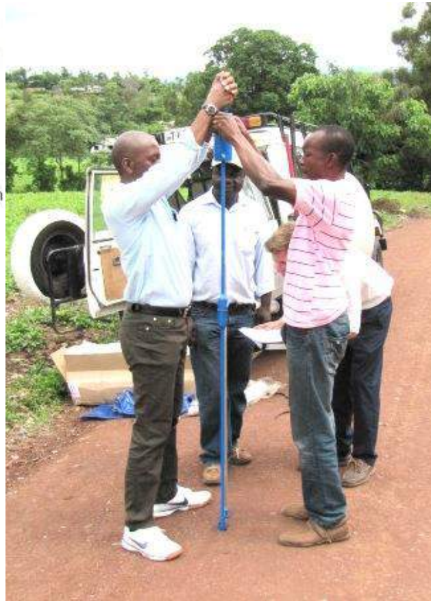
DCP test in process
