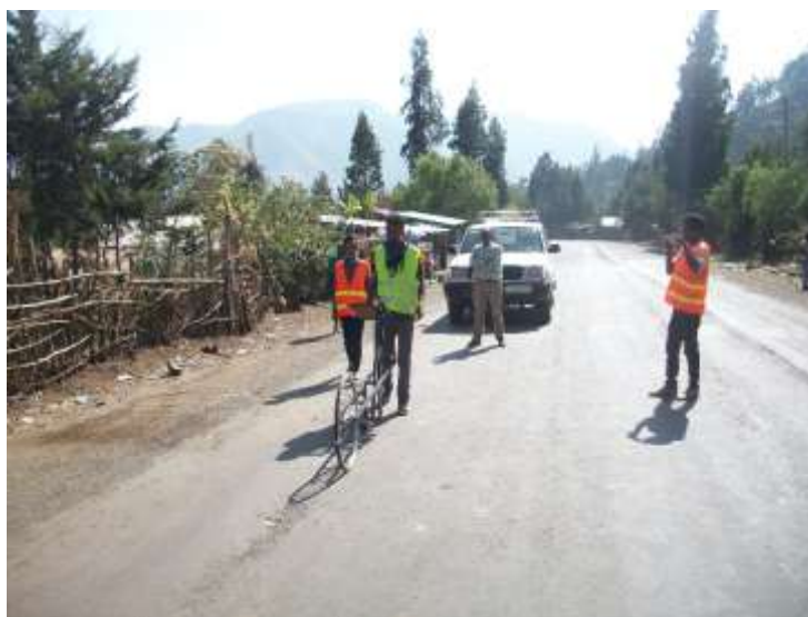
Figure 4-4: roughness measurement using MERLIN for Gerado Otta seal trial section
