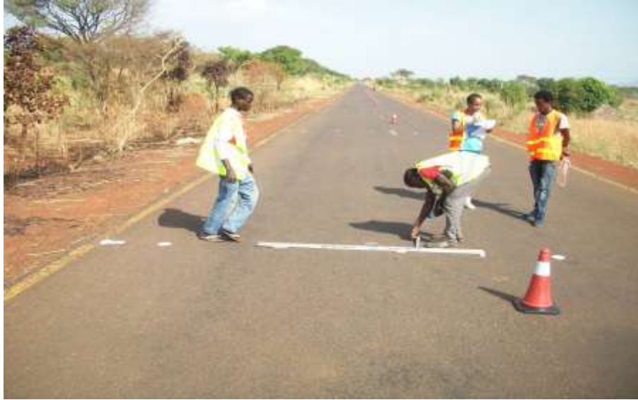
Figure 2-2: Rut depth measurement using 2m standard straight edge and measuring wedge.
