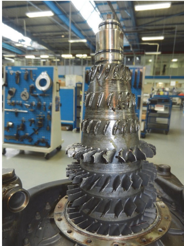
Figure 11 Right engine axial compressor
