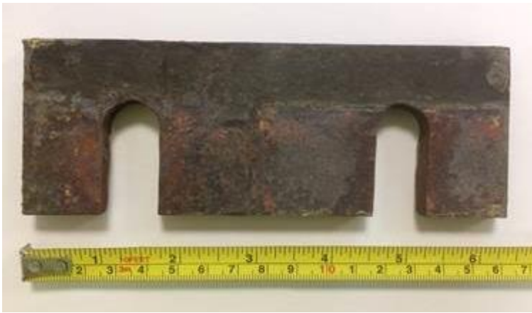
Photo 2 Original slotted shim
