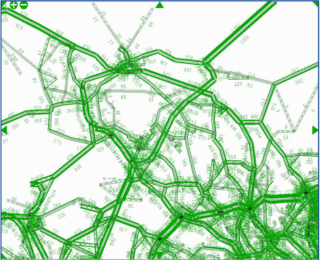
Figure 3 Model Traffic Flows AM 8-9 (Actual Flows, All Vehicles. pcu)
