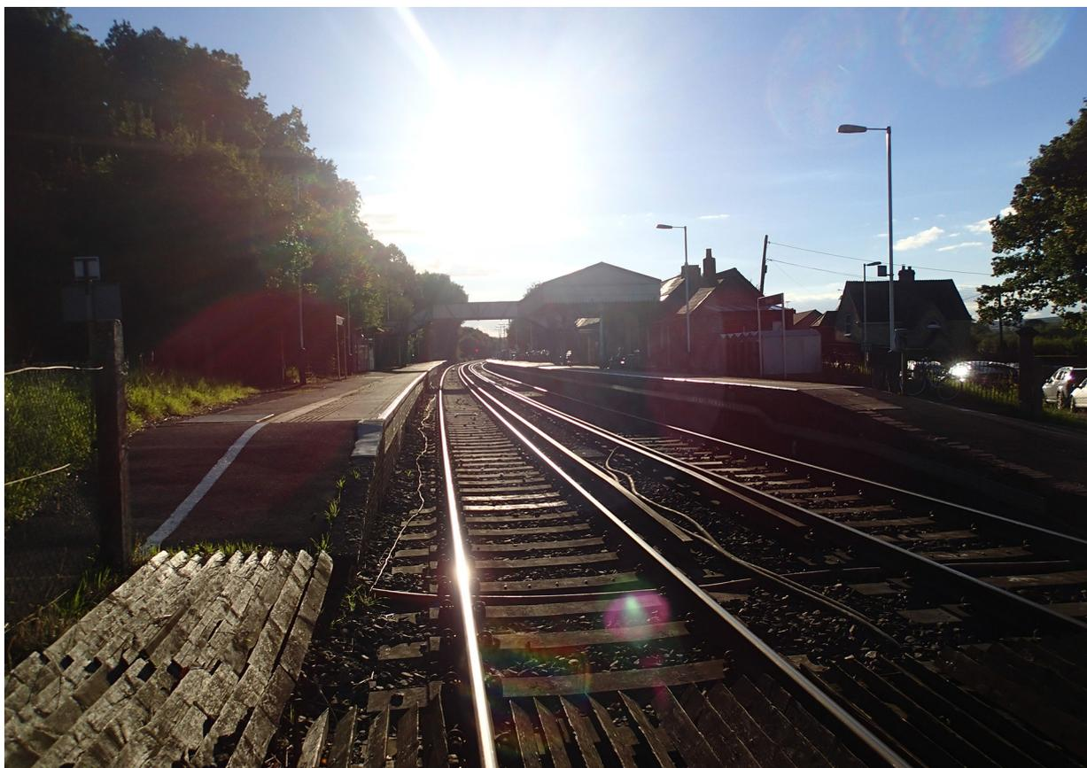
Figure 13: view from the southern end of the crossing decking, taken at the same time of day as the accident, showing the effect of sun glare
