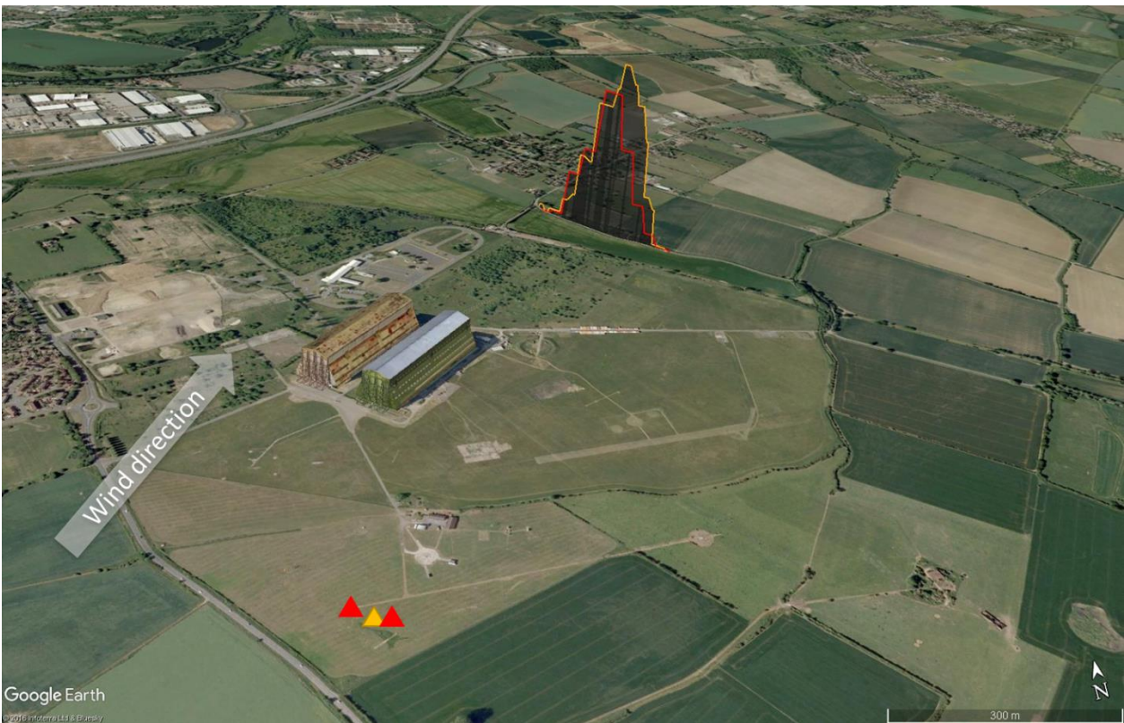
Figure E4.10 Release 10 gas release points, wind direction and monitoring route. Transect DTU 10.6 (Google Earth 2017)
