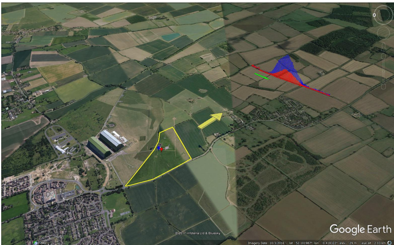
Figure E4.3 Release 8 gas release points, wind direction and monitoring route. Transect UOS 8.1 (Google Earth 2017)
