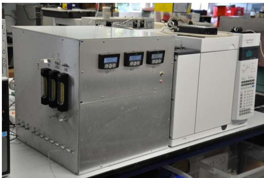
Figure 8: GC-ECD sample module (left), containing Nafion drier, valves and electronics, and the GC oven and ECD detector (right) (Met Office, 2012).
